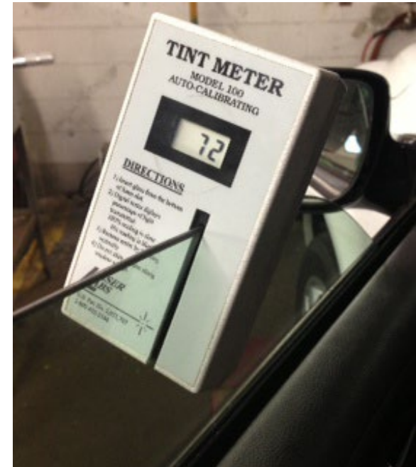
Light transmittance reading of factory glass with no aftermarket tint installed. Note: reading must be 70 or above to be approved.
